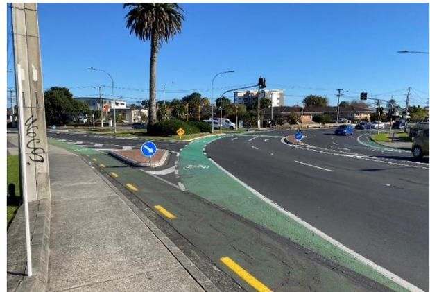
Figure 3-6: Station Road / Wyllie Road intersection with left turn slip lane into Wyllie Road
