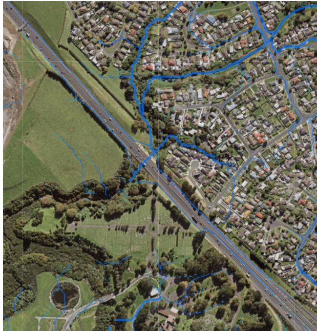
Figure 2-3: Example of Overland Flow Path shown as dashed (2000m 2 -4000m 2 ), thin (4000m 2 -3ha) and thick (>3ha) blue lines according to the contributing catchment area.
