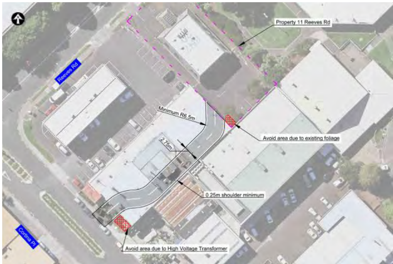
Figure 77: 11 Reeves Rd temporary access during construction
