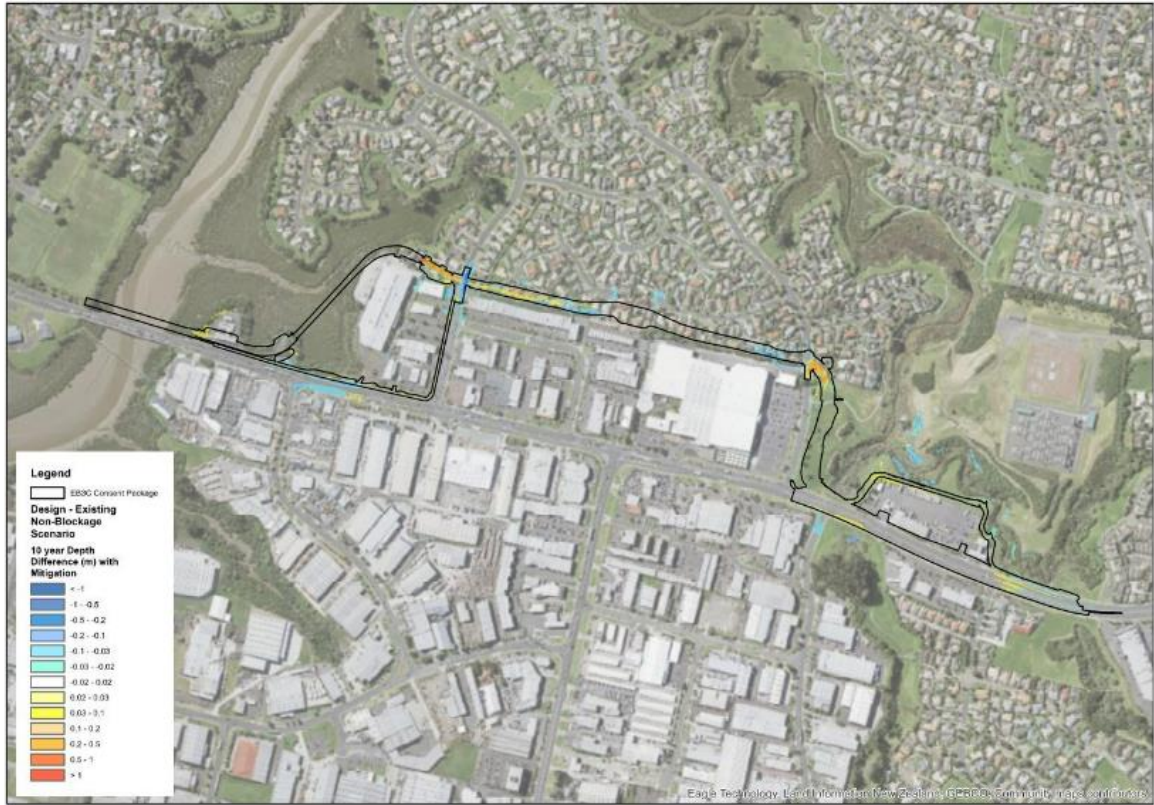
Figure 37. EB3C design case with mitigation 10-year flood depth difference
