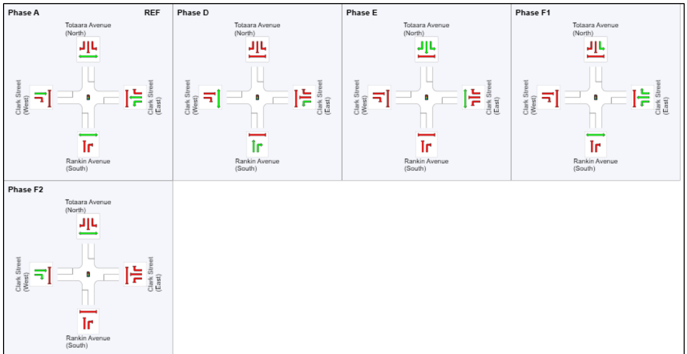
Figure 2-8: SIDRA intersection - Clark Street / Rankin Avenue / Totara Avenue – adopted phasing arrangement
