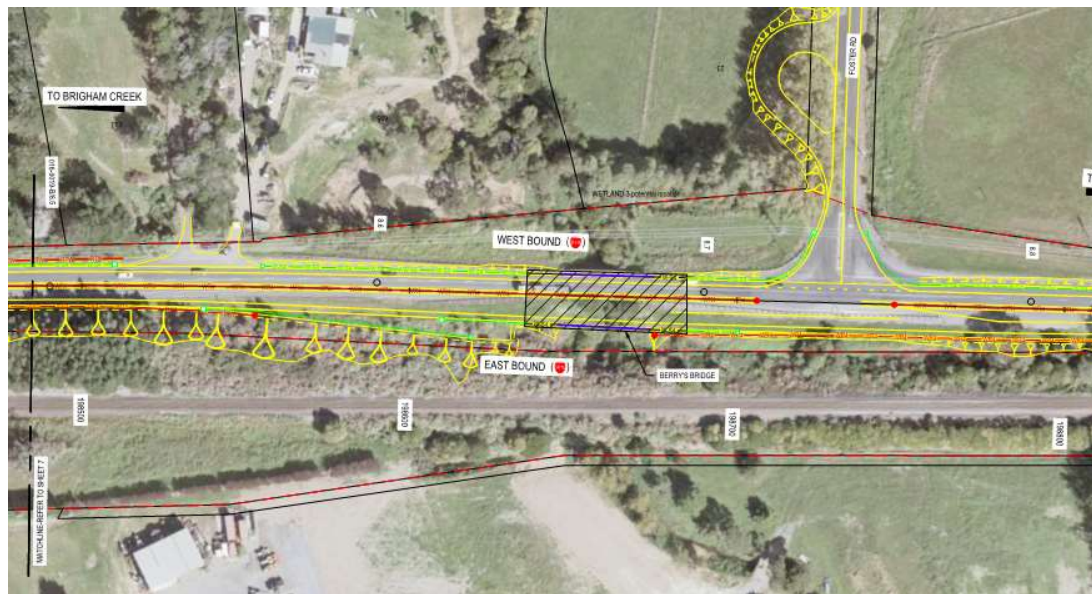
Figure 1: Section of SH16 to be widened
