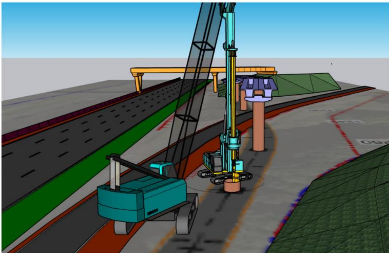
Figure 3-6: Pile being installed with support crane
