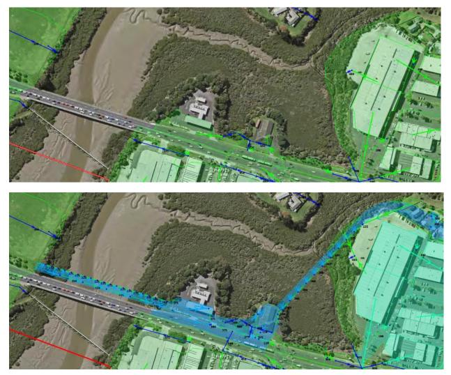
Figure 5: EB3C – EB4 base model (top image) and EB3C – EB4 design model (bottom image) with additional sub-catchments added to Ti Rakau Drive busway bridge.
