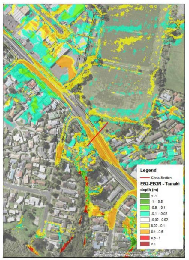
Figure 8: EB2-EB3R - Tamaki depth difference at Ti Rakau Park.
