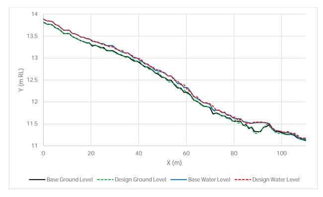
Figure 6: Ground level and water level long section at Cindy Place shown in Figure 7.
