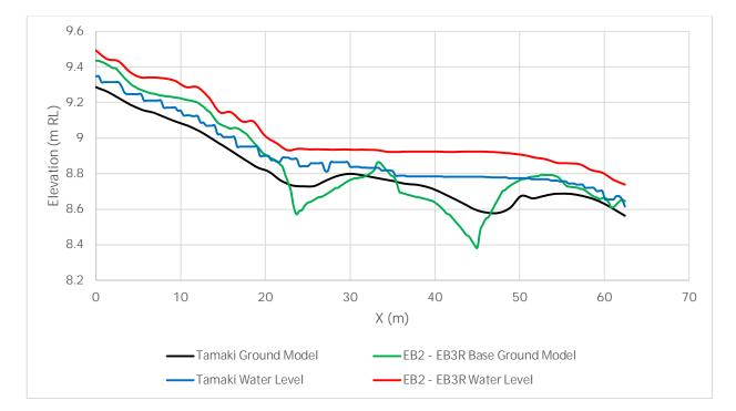
Figure 9: Cross section of Tamaki and EB2-EB3R ground models and water levels.
