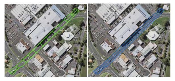
Figure 4: Flyover sub-catchments loaded to downpipes (green) and flyover sub-catchment to be loaded to the pipe network to the west in the detailed design stage (blue).
