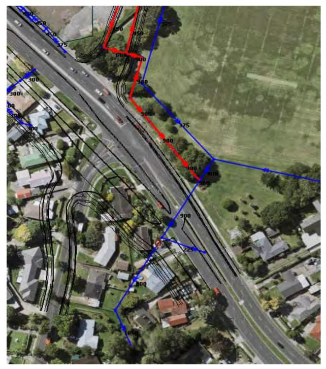
Figure 10: WRR design network highlighted in red connecting to the existing pipe network shown in blue.
