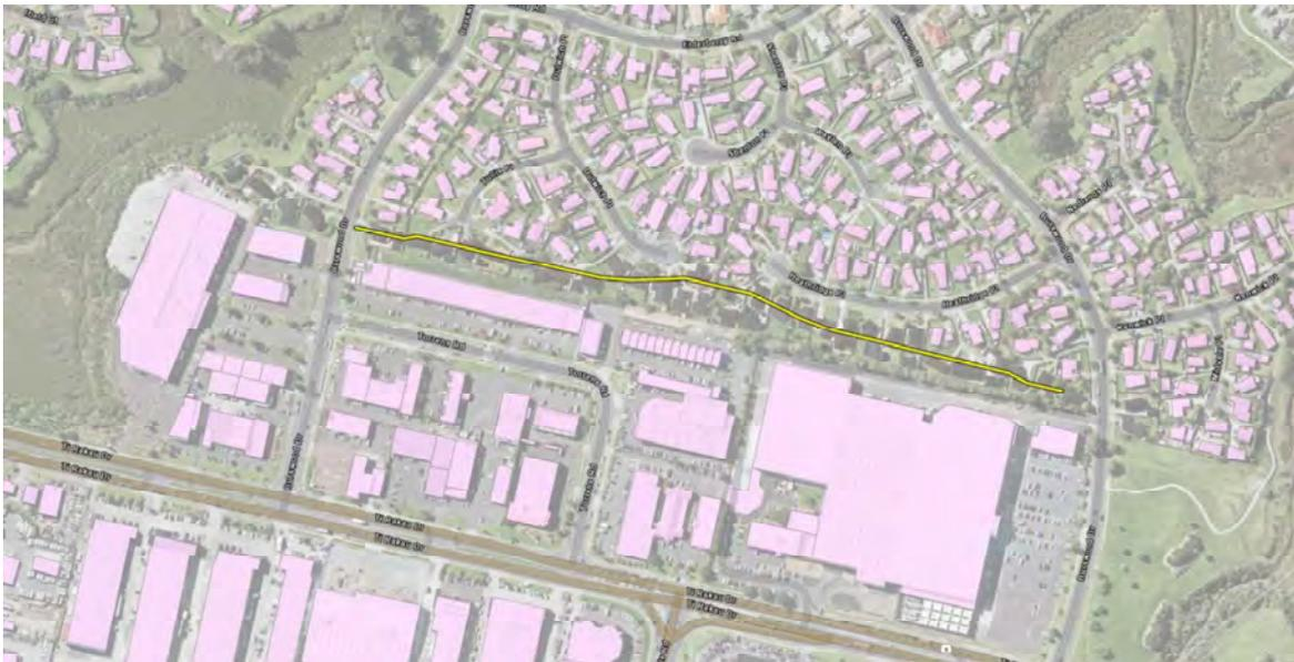
Figure 5-1 Noise barrier proposed by Project design team
