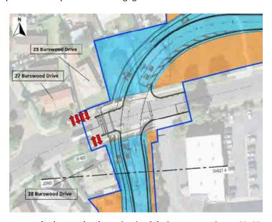
Figure 67: Property accesses (red arrows) to be maintained during construction at 25, 27 and 28 Burswood Dr
