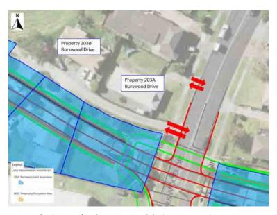
Figure 68: Property accesses (red arrows) to be maintained during construction at 203 Burswood Dr
