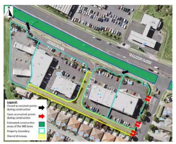
Figure 71: 347 Tī Rākau Drive, 2 and 12 Amera Place, 371 Tī Rākau Drive vehicle access points during construction
