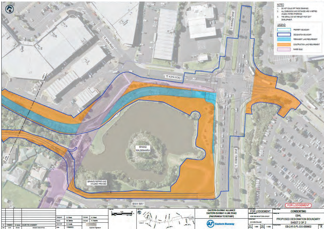
Figure 20: EB4L Designation Plan which shows the permanent and temporary land required for EB4L
