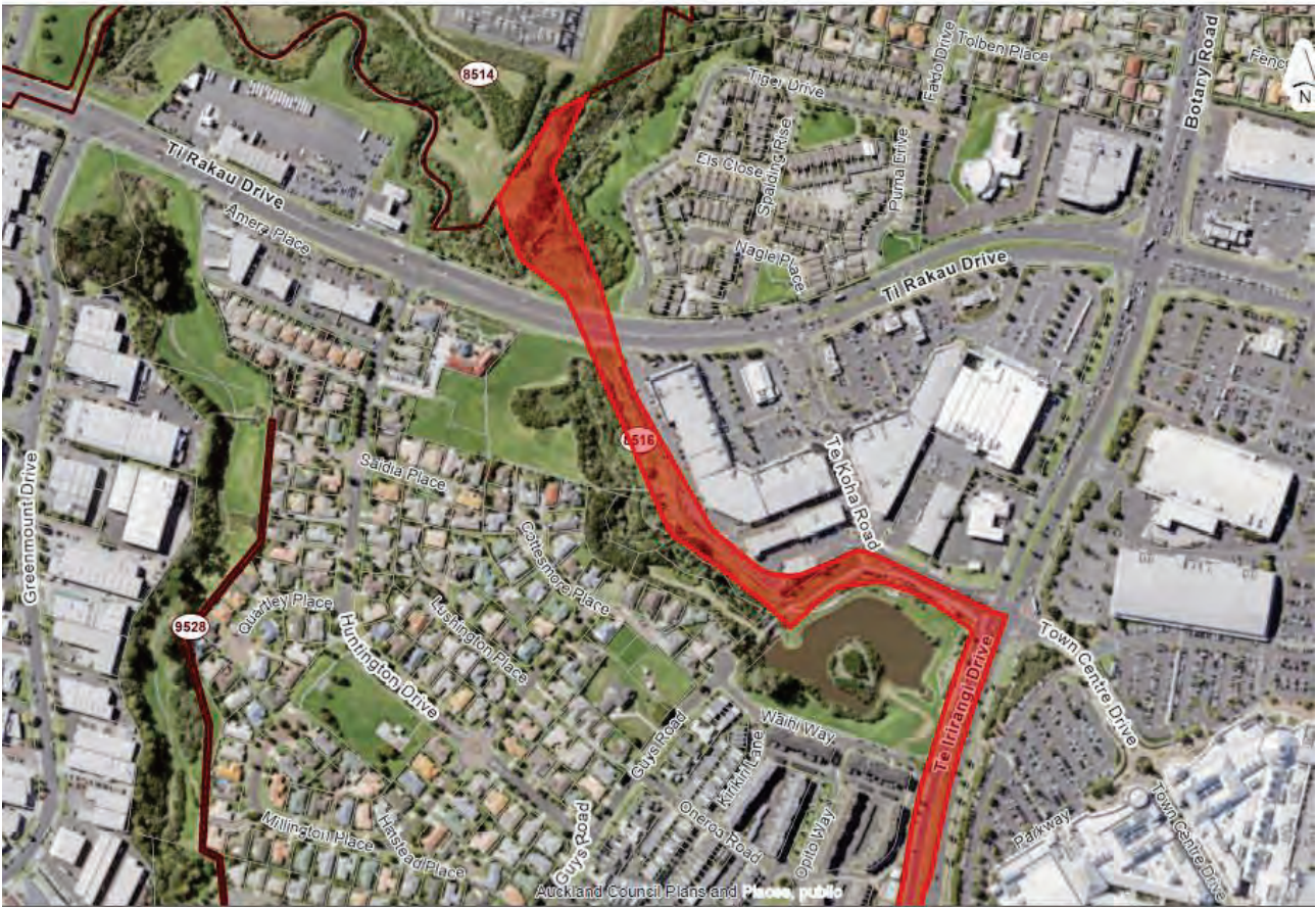
Figure 14: Extent of the underground electricity transmission of a 220kV cable located within the Guys Reserve and Whaka Maumahara Reserve
