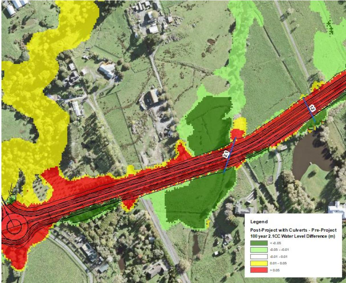
Figure 6. Location Plan Area 3 showing the flood results with the addition of a 2100mm culvert.
