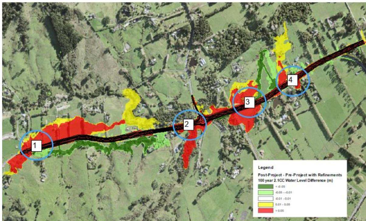
**Figure 1. Predicted post Pine Valley Road upgrade future 100yr 2.1° climate change water level difference and location plan of culvert amendments.**
