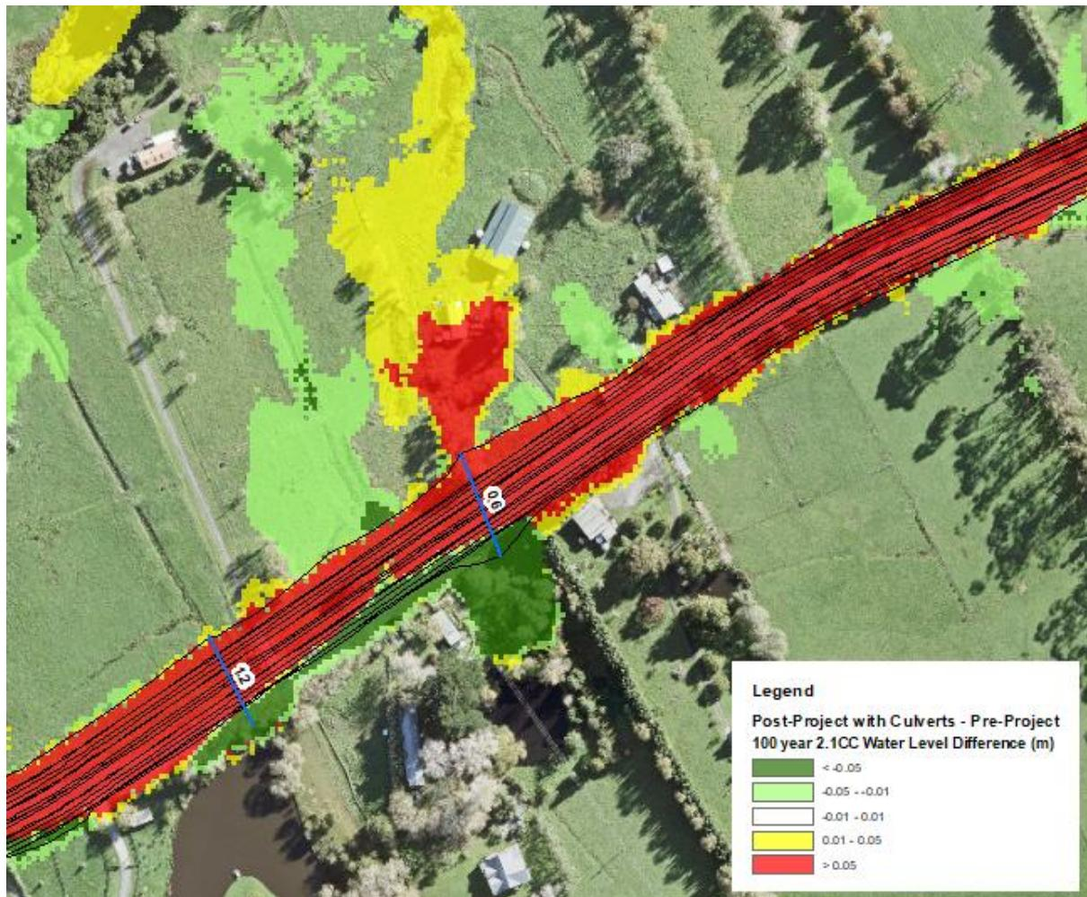
Figure 7. Location plan area 4 showing the Post-Project flood results with two 600mm culverts.
