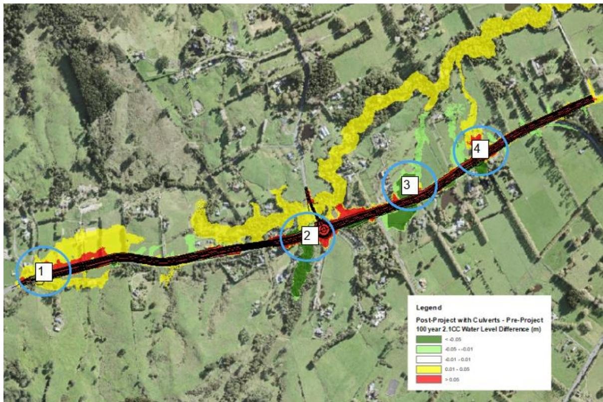
**Figure 2. Predicted post Pine Valley Road with amended culverts 100yr 2.1° climate change water level difference and location plan of areas discussed in detail.**
