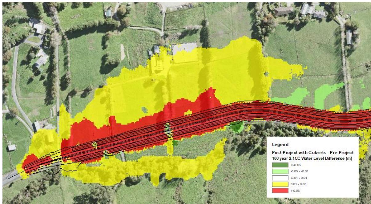
Figure 3. Area 1 location showing results with terrain openings to represent culverts.
