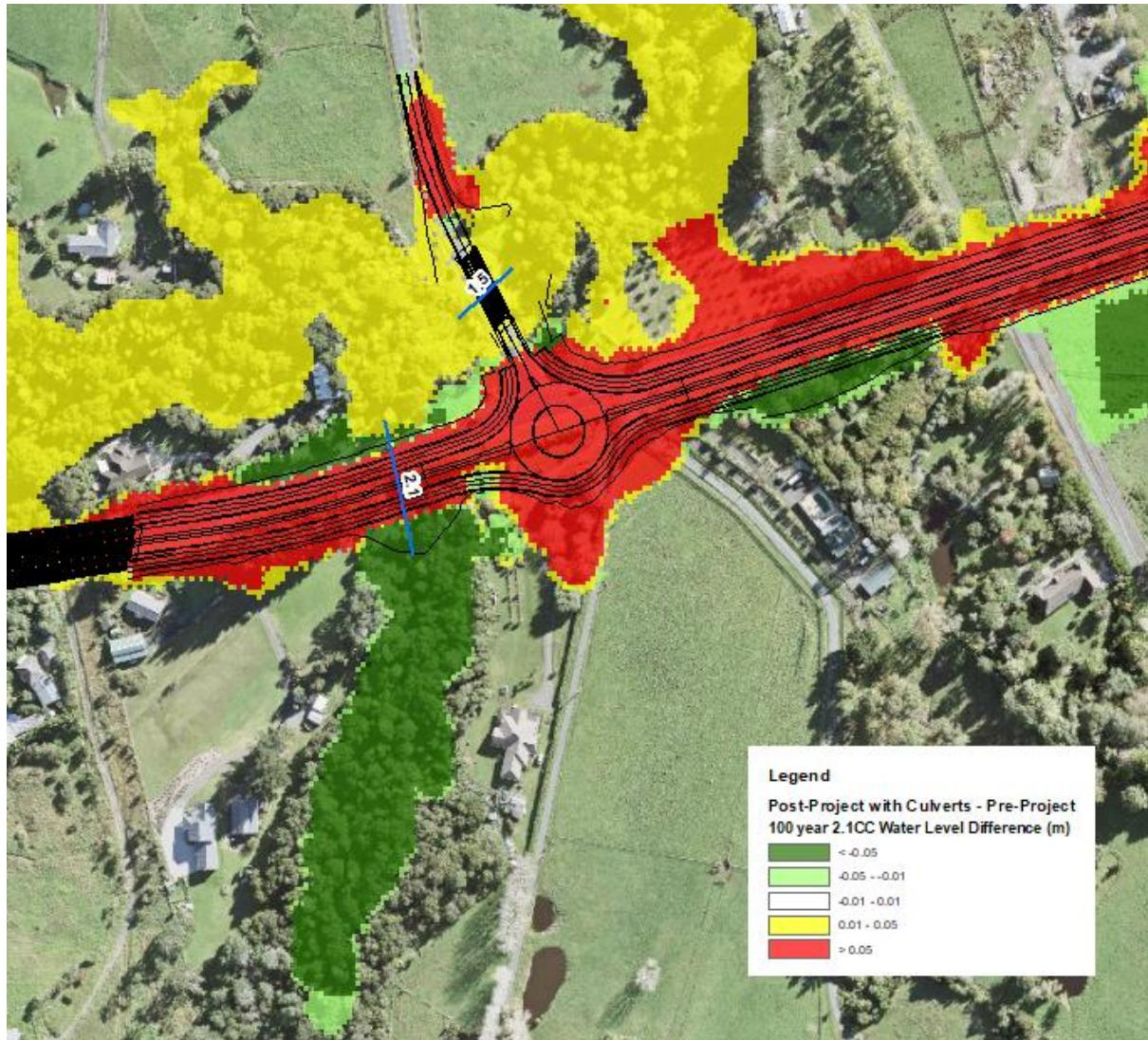
**Figure 5. Location Plan Area 2 showing the post Project flood results with the addition of a 2100mm culvert.**
