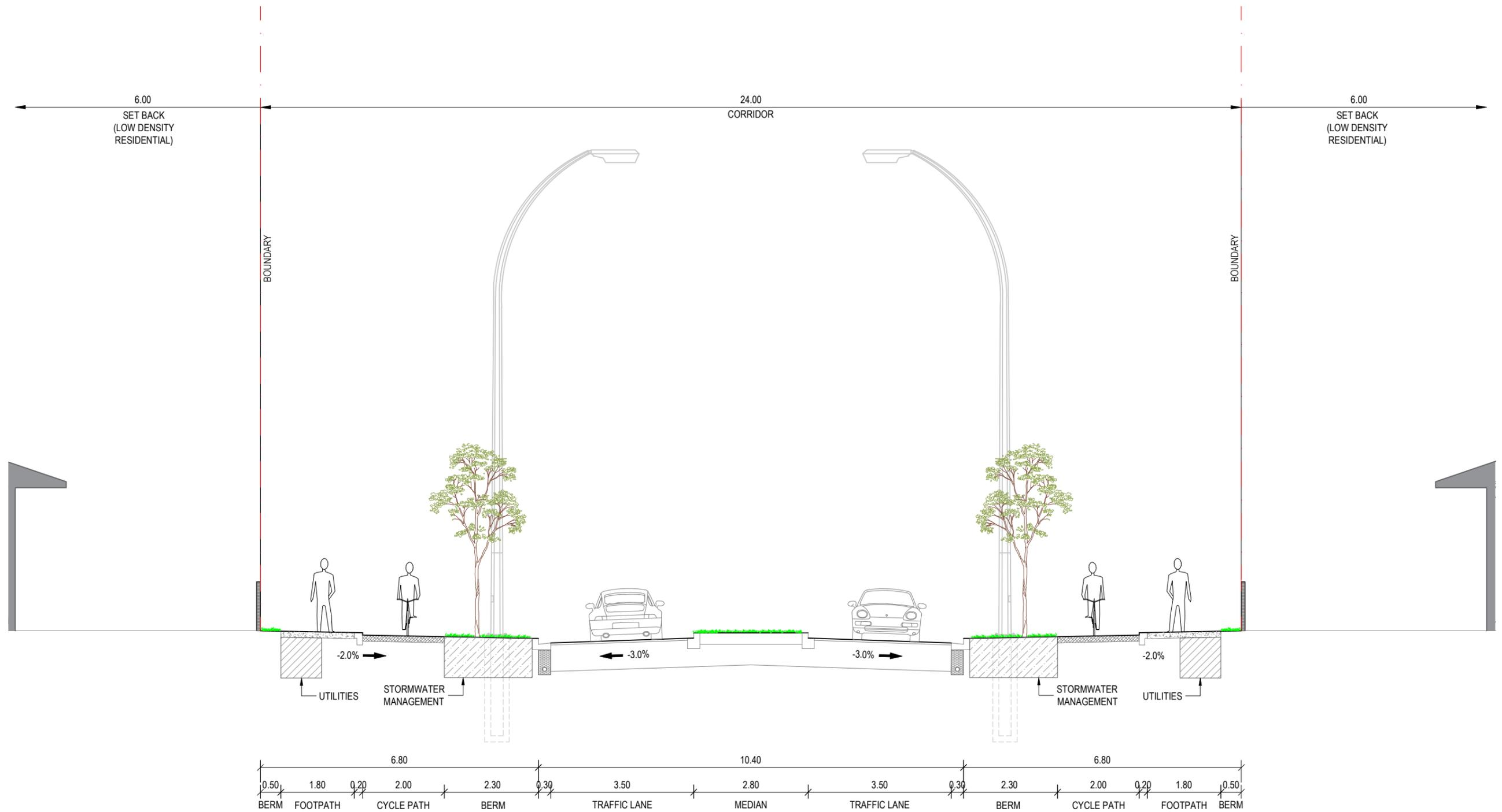
Standard cross section to be used for a 2 lane arterial.
