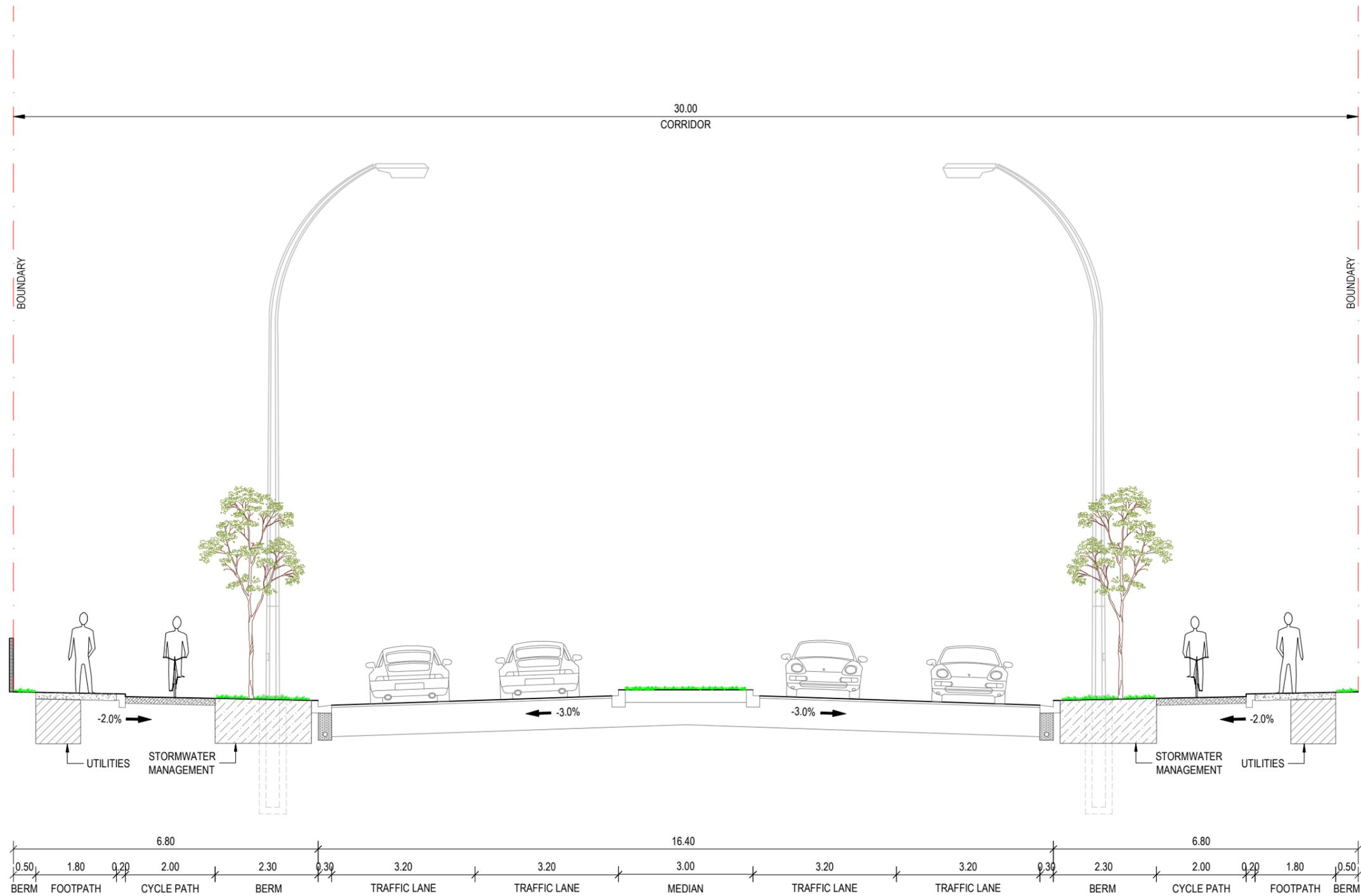
Standard cross section to be used for arterials with no strategic PT function. Four lane cross section with FTN (below) should also be used for engagement to demonstrate that the additional lanes could be used for Public Transport in the future.
