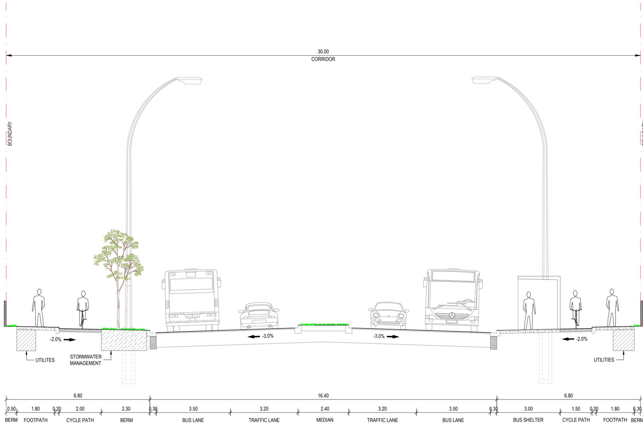
This shows both a station scenario (right side) and a mid-block corridor scenario (left side). The majority of the corridor will be mid-block, so the left side cross section should be used and duplicated in both directions (so that the cross section is symmetrical). This will simplify the design process.
