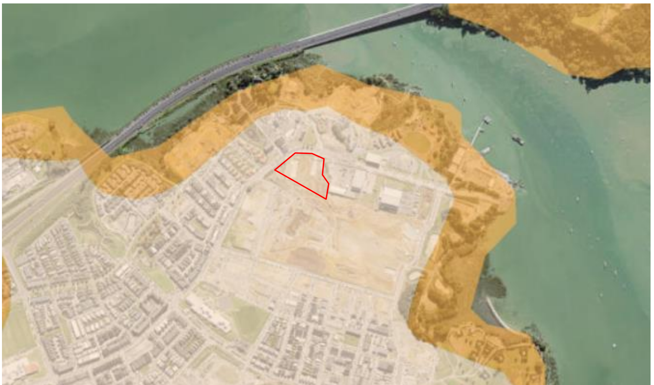
Figure 2. Geology of the site and surrounds: pale yellow indicates Puketoka Formation; orange indicates East Coast Bays Formation. (Source: GNS Webmap).
