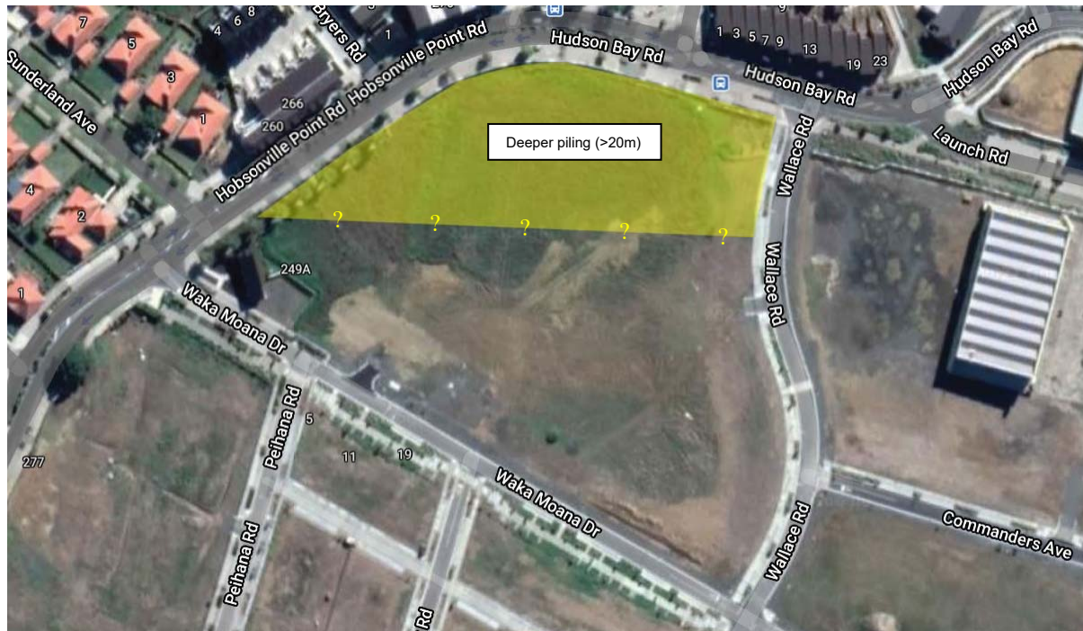
Figure 5-1 – Area of site likely to require pile depth of > 20m bgl – possibly up to 30m
