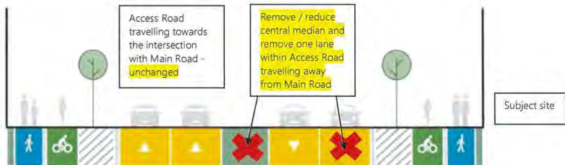
Figure 1-7: Indicative Access Road Upgrade cross section for urban section
