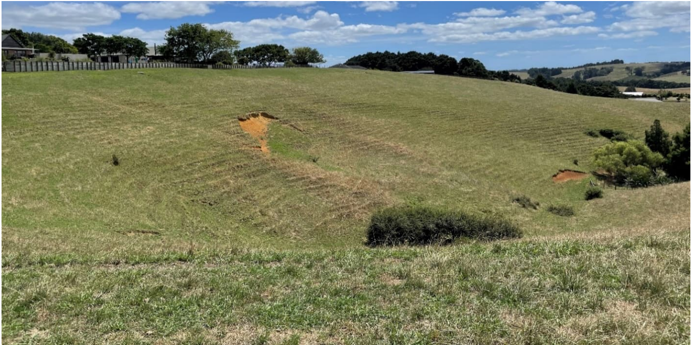
Photo 6: Arcuate slip located west of the gully, below the ridgeline.
