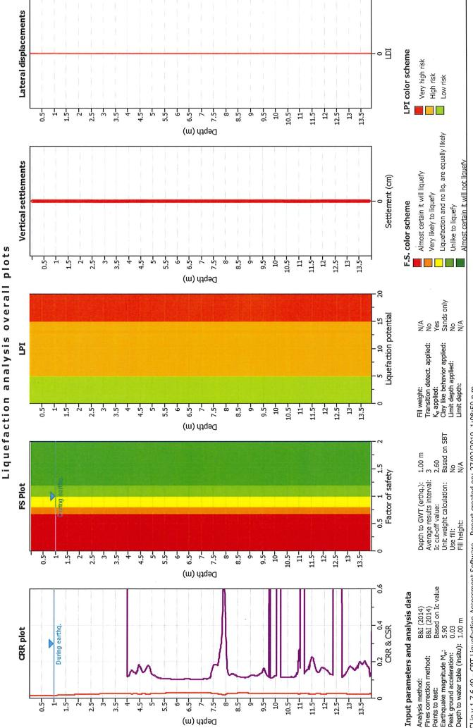
CLiq v.1.7.6.49 - CPT Liquefaction Assessment Software - Report created on: 27/02/2019, 1:08:59 p.m. Project file: \\LGSV01\Shared Folders\Company\PROJECTS\J00784 116 WAIHOEHOE RD DRURY\3 FIELD DATA & BOREHOLES LOGS\3.2 FIELD & BOREHOLE RECORDS\CPT'S\CPT analyses\J00784\_190227\_SLS.dc
