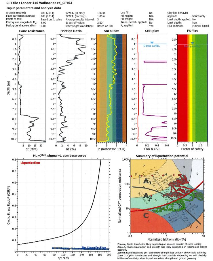
CLiq v.1.7.6.49 - CPT Liquefaction Assessment Software - Report created on: 27/02/2019, 1:09:00 p.m. 5 Project file: \\LGSV01\Shared Folders\Company\PROJECTS\J00784 116 WAIHOEHOE RD DRURY\3 FIELD DATA & BOREHOLES LOGS\3.2 FIELD & BOREHOLE RECORDS\CPT'S\C
