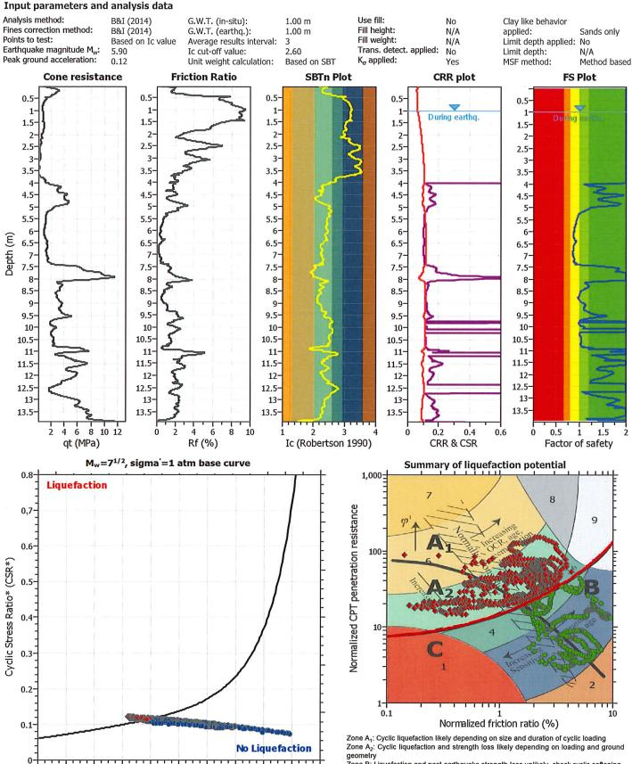
Zone B: Liquefaction and post-earthquake strength loss unlikely, check cyclic softening Zone C: Cyclic liquefaction and strength loss possible depending on soil plasticity, brittleness/sensitivity, strain to peak undrained strength and ground geometry
