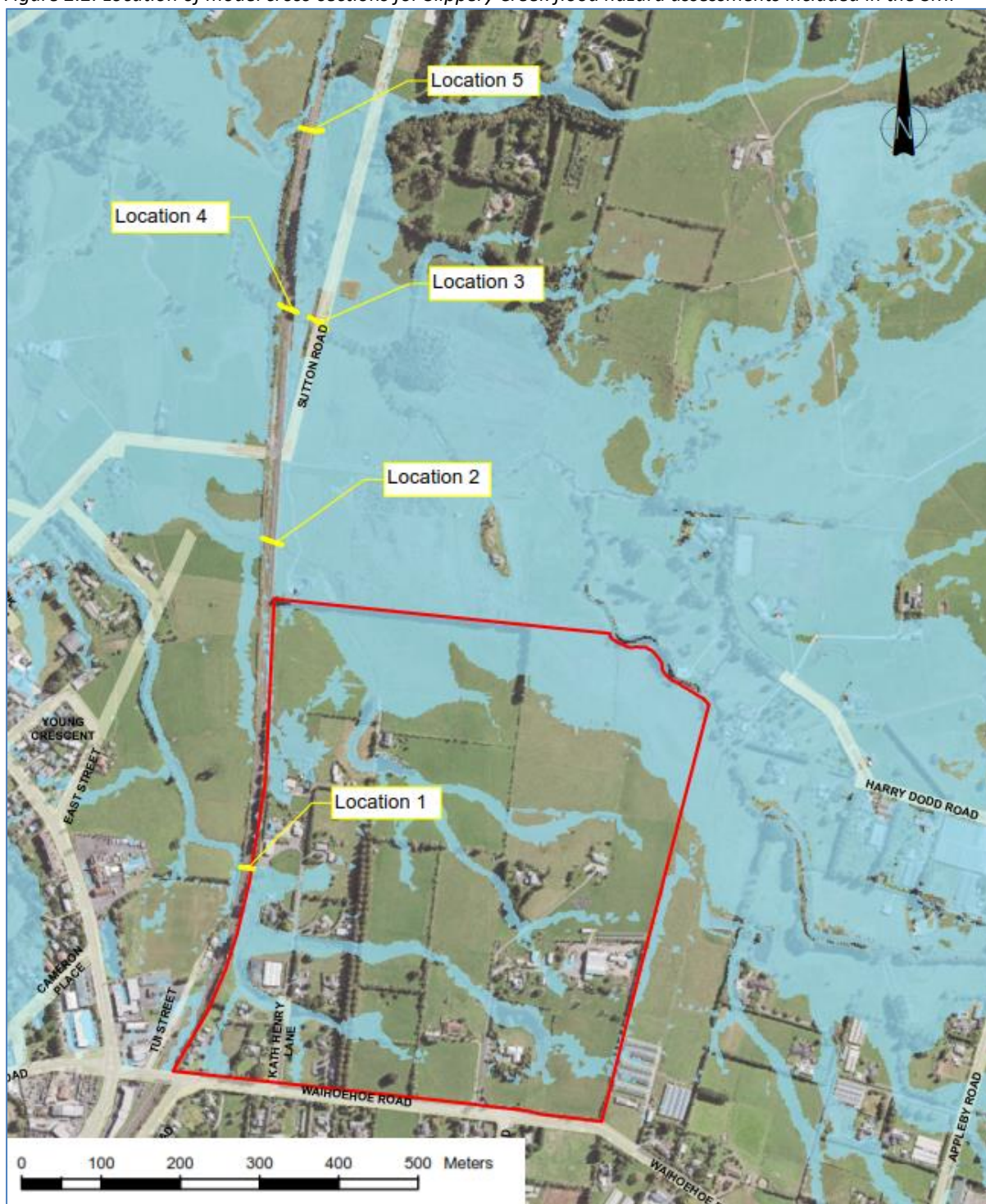
Figure 2.2: Location of model cross-sections for Slippery Creek flood hazard assessments included in the SMP
