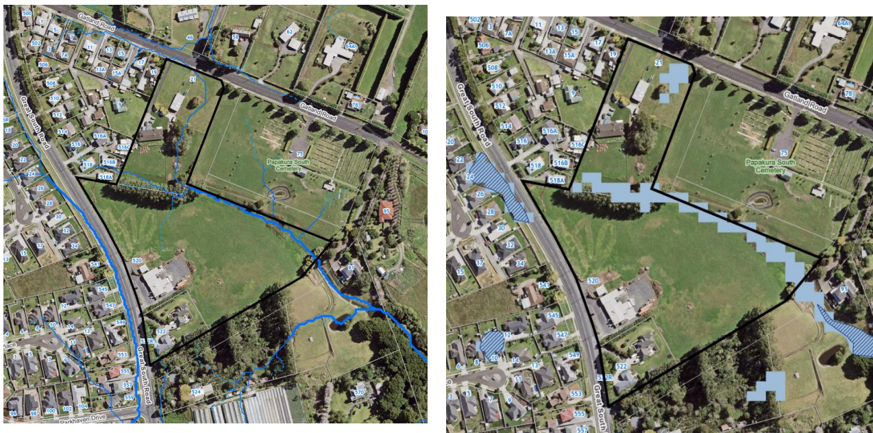
Figure 2.8: Overland flow paths, flood plains and flood prone areas
