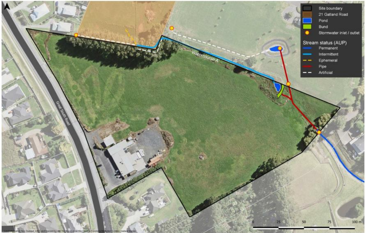
Figure 1.2: Existing private stormwater drainage within the PCA (Freshwater Solutions, 2020)
