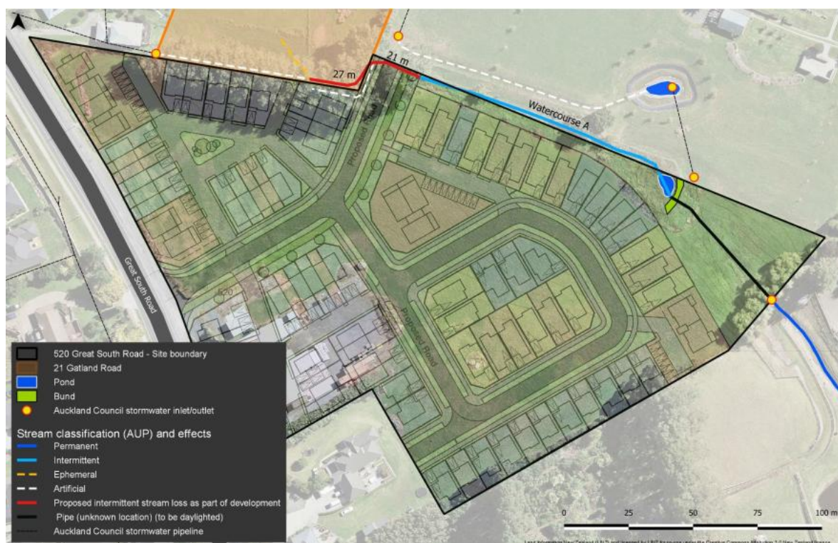
Figure 6.3: Proposed stormwater drainage (Freshwater Solutions, 2020)
