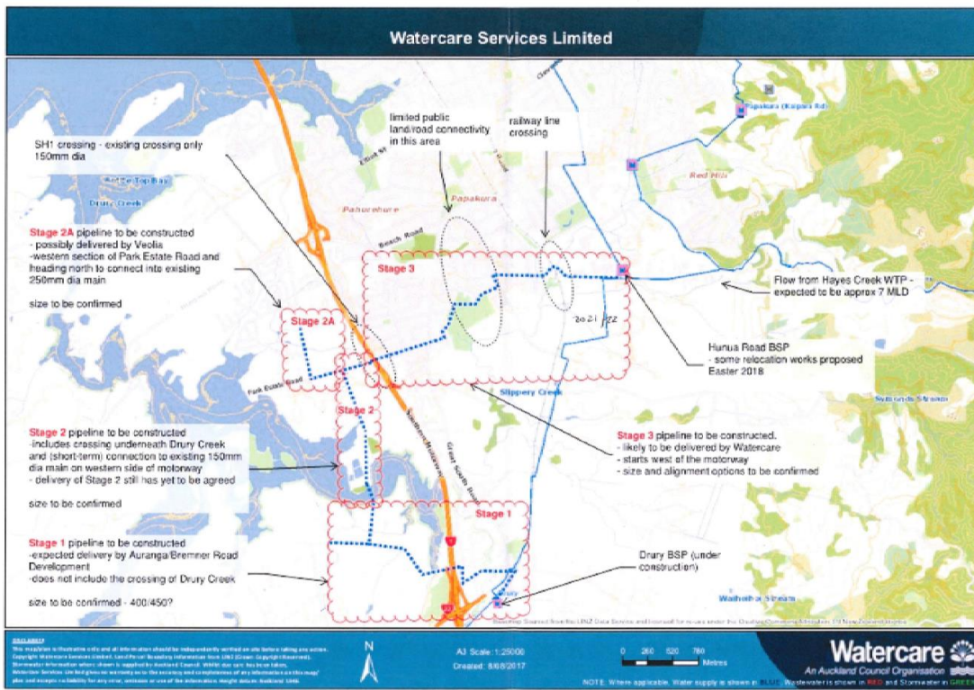
Figure 5 – Watermain servicing for the southern Hingaia area.
