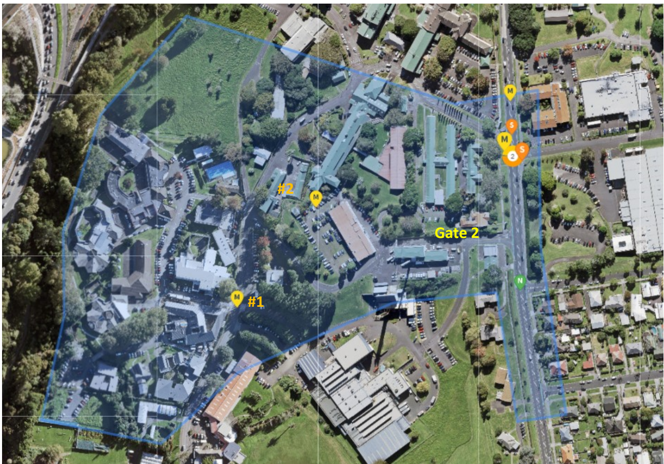
Figure 8: CAS results - Crash distribution and severity (S=severe injury crash; M=moderate injury crash; N=non-injury crash)
