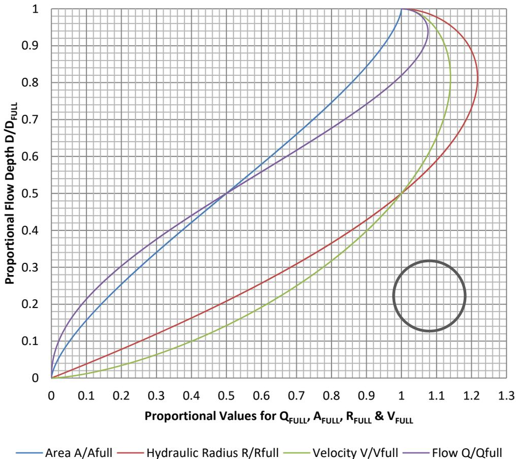
The flow depth and velocities are calculated to the maximum flow, not full pipe flow. This will calculate the maximum flow velocity for any flow rate, giving a small margin of error for flow depths greater than 91%.
