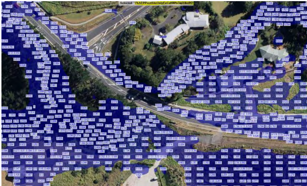
Figure 7: 1% AEP Post-Development Flood Depths (PCA) With Climate Change
