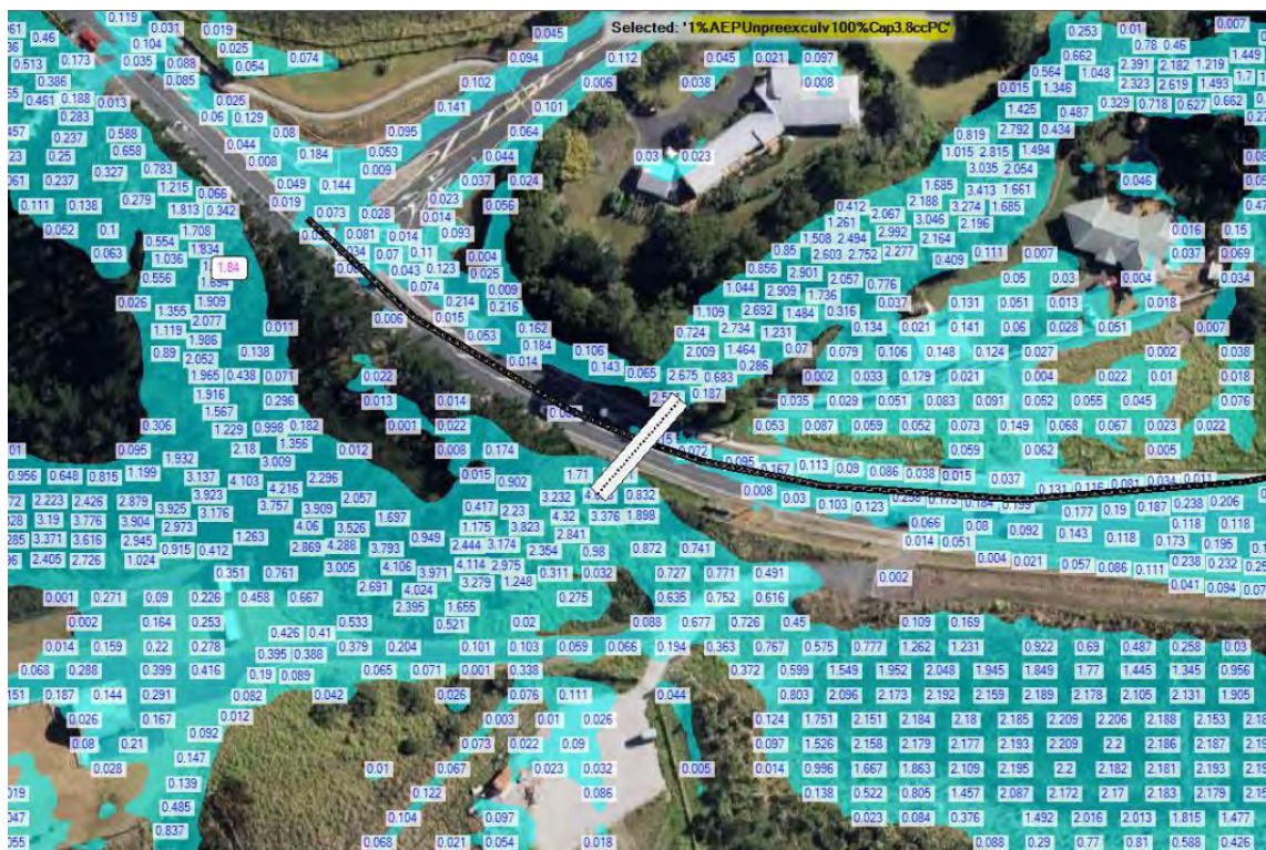
Figure 6: 1% AEP Pre-Development Flood Depths with Climate Change
