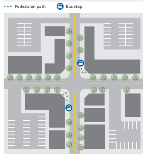
Figure 7 – Pedestrian-oriented urban design features buildings with fine-grained active frontages built right to the street and with parking tucked behind or provided underground.
