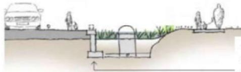
Concrete wall to support side of device if adjacent to road
