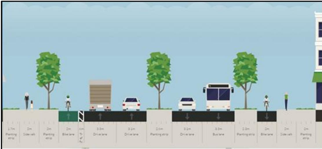
**FIGURE 9: 32M TYPICAL ARTERIAL CROSS SECTION**
