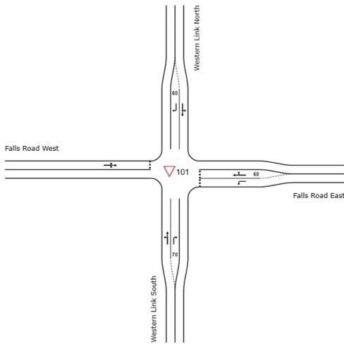
**FIGURE 11: LAYOUT FOR SOUTHERN END INTERSECTION - PRIORITY 2036**
