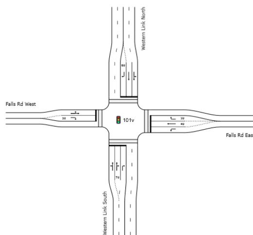
**FIGURE 14: LAYOUT FOR SOUTHERN END INTERSECTION - SIGNAL 2046**
