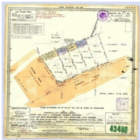
Figure 40: 1955 Deposit Plan showing the further subdivision of part of the land (part lot 2 and lot 3 of above) on the corner of Remuera and Upland roads into five lots, upon which four shop buildings were subsequently built (present-day 610-618) (DP 43480, LINZ records).
