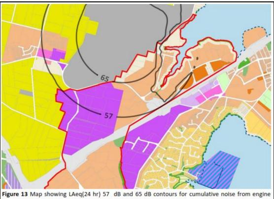
**Figure 13** Map showing LAeq(24 hr) 57 dB and 65 dB contours for cumulative noise from engine testing of the B757, C130 and P3 aircraft conducted at Whenuapai Airbase over a 'worse case' seven day rolling time period recorded during the 60 day survey of engine testing conducted in 2016.
