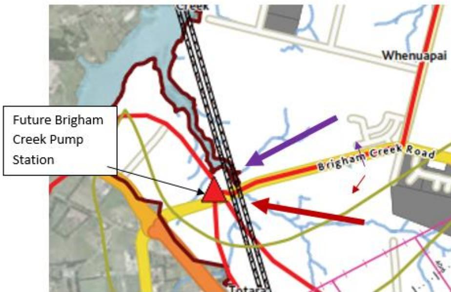
**Figure 8: Future stand-alone wastewater pump station and rising main**
