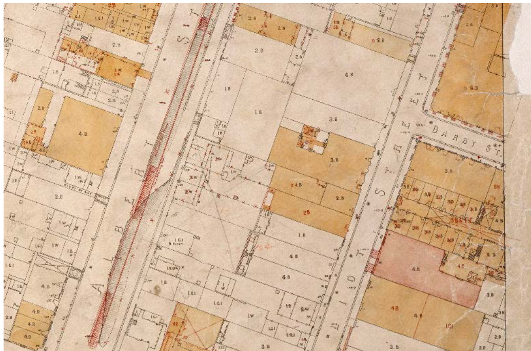
Figure 1: Detail of map of central Auckland 1908 showing the building on the corner of Elliott and Darby Street. The notation 3B refers to the building being three storeys and brick
