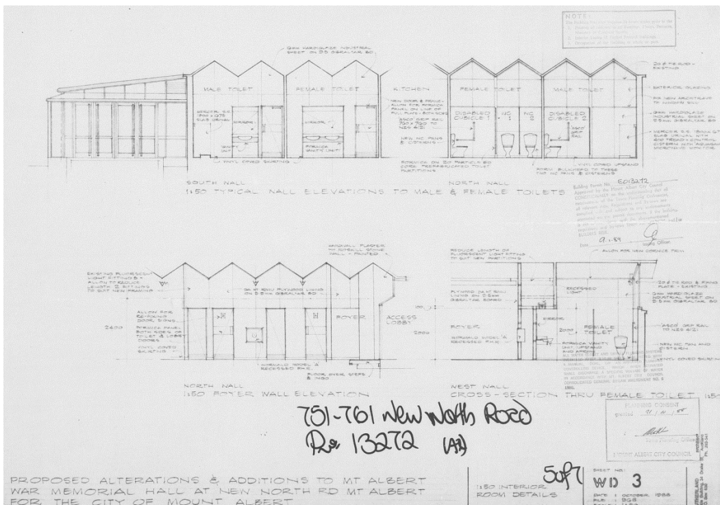
Figure 56: Drawings show the additions of the entrance hall and alteration to the rear building. Auckland Council Archives microfilm, June 1988.
