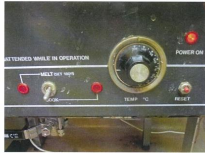
Figure 4 - Oven Temperature safety cut-out switch
