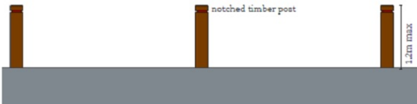
Figure 13 - Fencing Detail 3 - Public Open Space - Conservation
