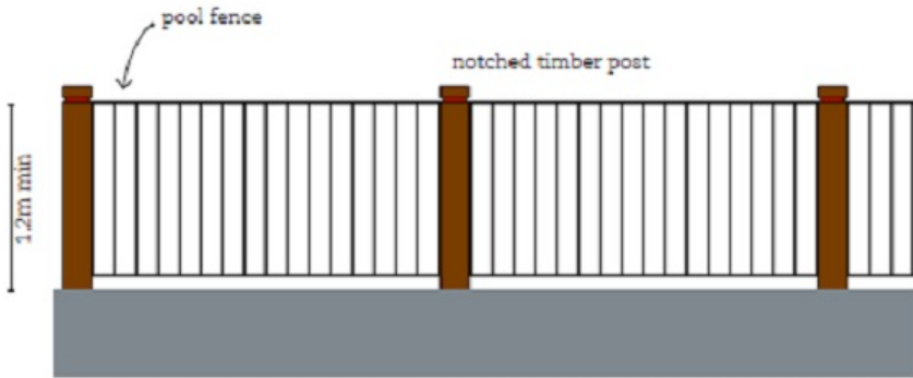
Figure 14 - Fencing Detail 4 - Green Infrastructure Zone
