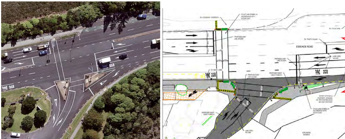
Figure 3.1: Existing (left) and proposed (right) intersection layout (Map source: Auckland Council GEOMAPS)
