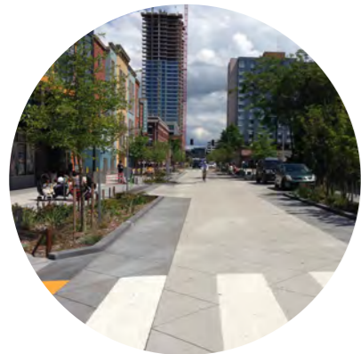
PC1-PEDESTRIAN CROSSING IN-SITU CONCRETE/ PAINT
