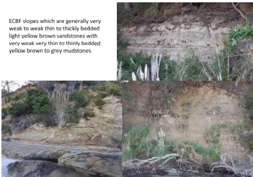
Figure 3-4: ECBF bedded mudstones and sandstones, dipping 06/180. Shown as 2 in Error! Reference source not found.
