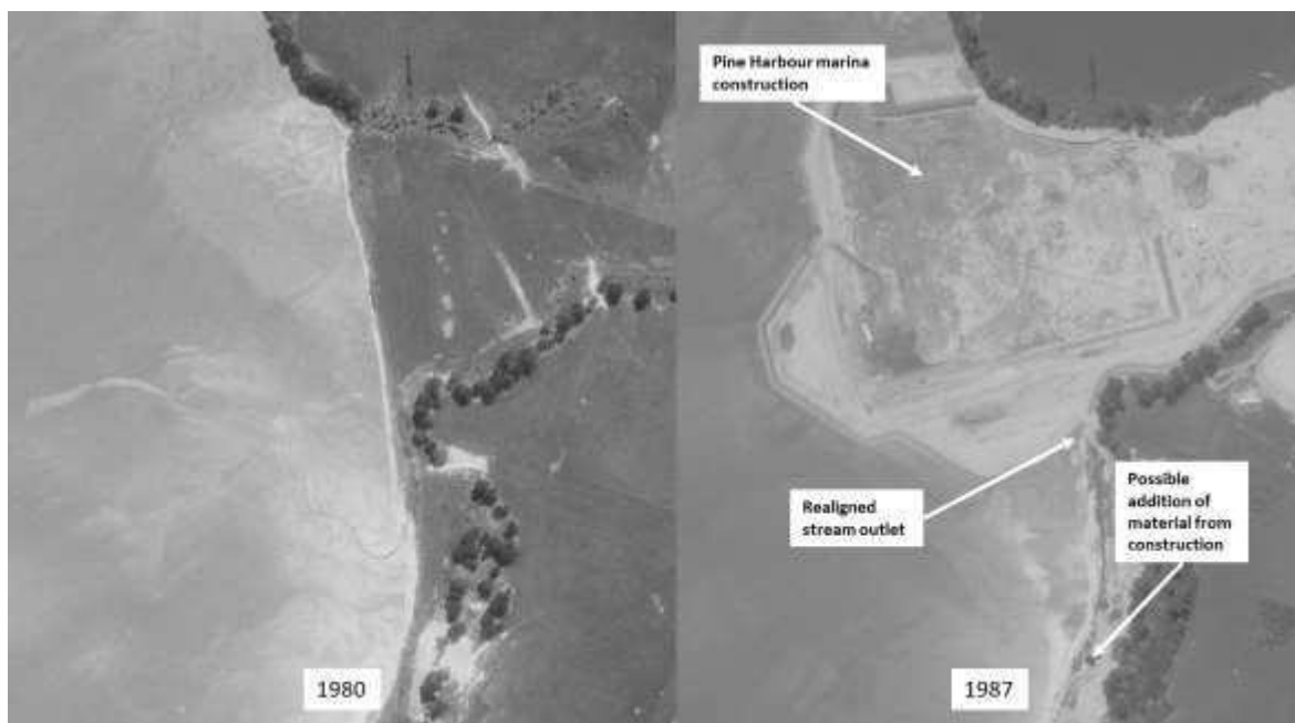
Figure 4-2: Comparison of 1980 and 1987 aerial photographs at the present location of Pine Harbour marina
