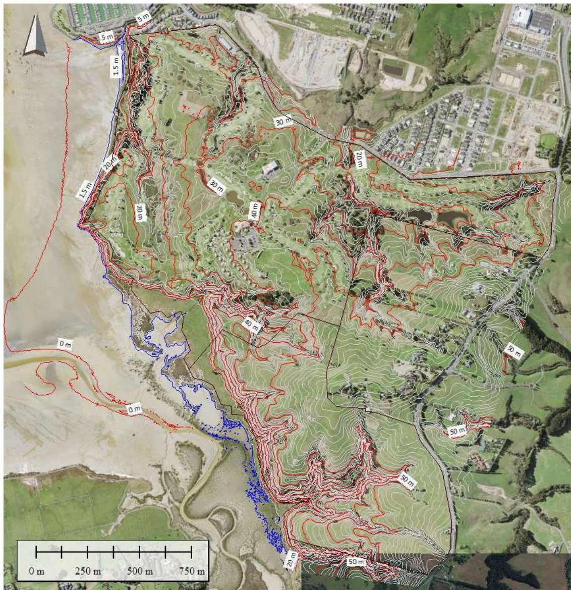
Figure 3-8: Site contours based off 2016 AC LiDAR data. Minor contours in grey, major contours in red, indicative MHWS level (m RL) in blue.
