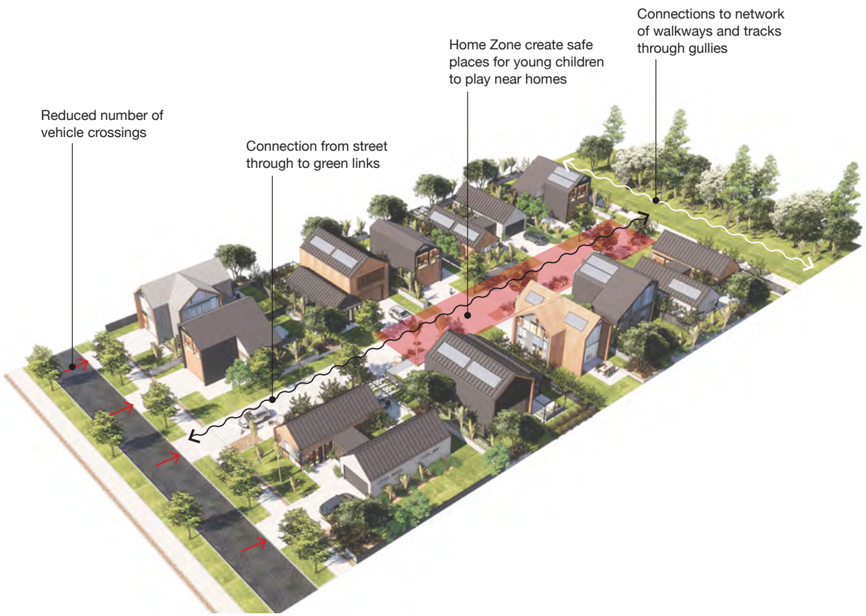
Figure 23. Illustration of home-zone - promoting connections to the wider walking and cycling network with safe, slow-speed streets
