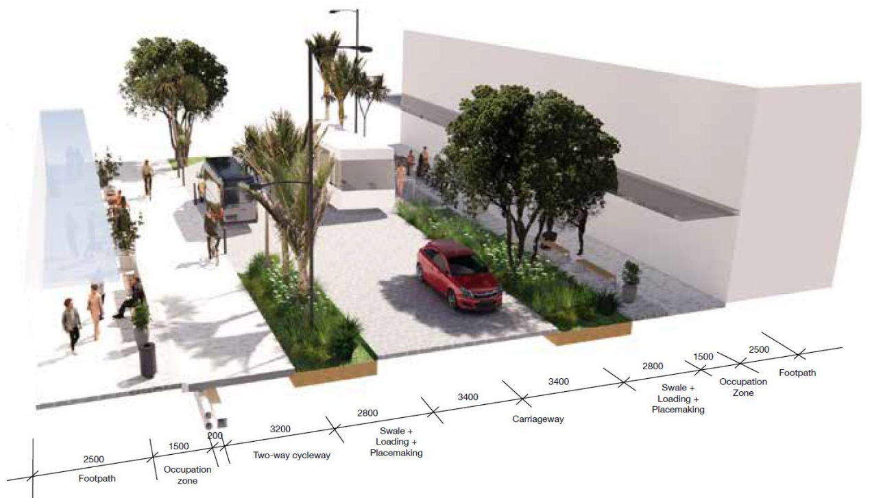
Figure 13. Street Cross-section: Primary Collector (Village Centre)
