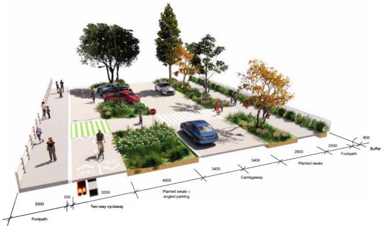
Figure 14. Street Cross-section: Primary Collector (School Zone)
