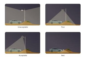
Figure 14 Lighting options for a parking area. Figure adapted from Witherington and Martin (2003)<sup>3</sup>.
