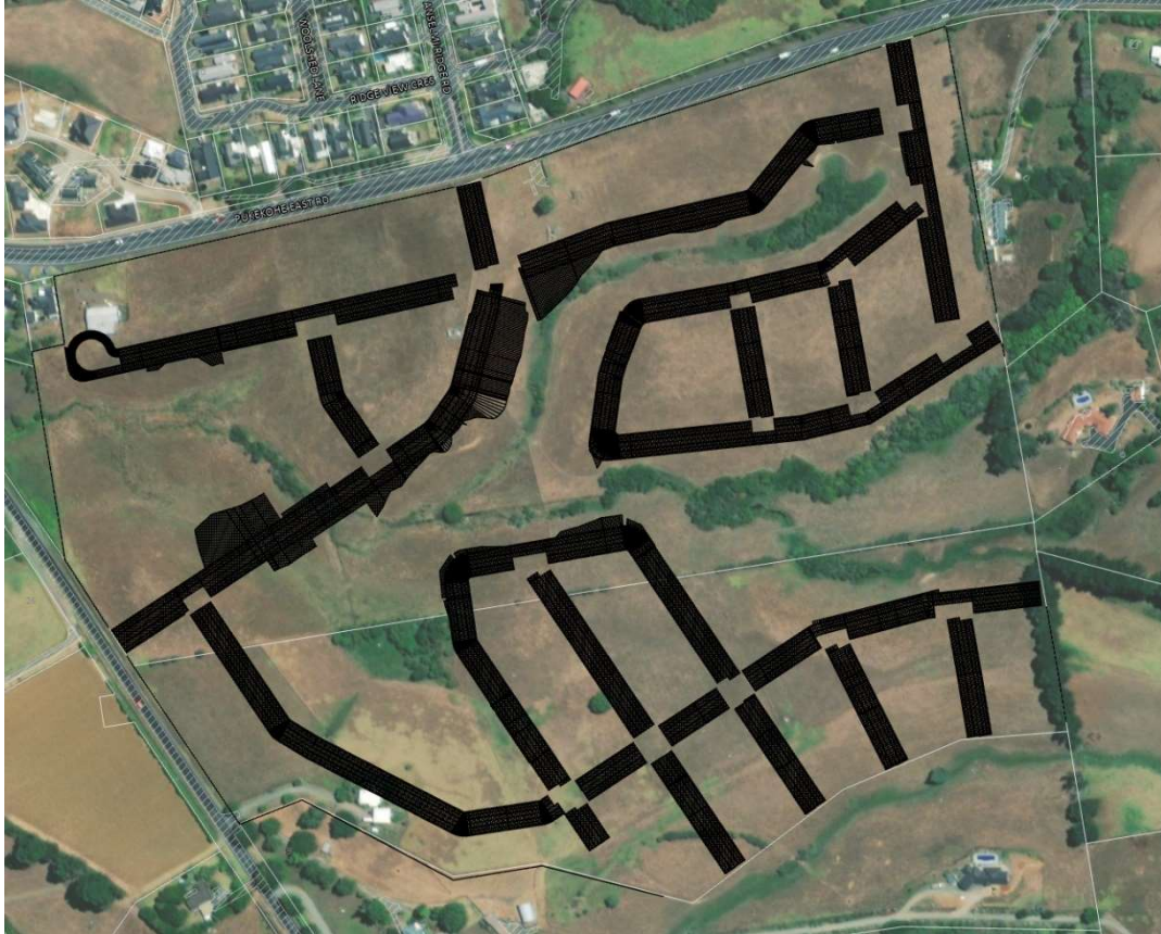
Figure 6 – showing the proposed roading layout of the site (refer to Concept Master Plan for details)
