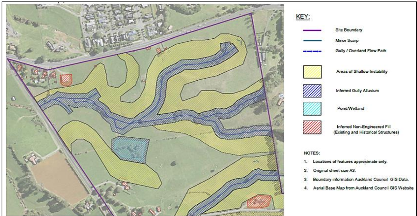
Figure 10 – Plan indicating the areas of instability across the Site. Source: Soil & Rock Consultants
