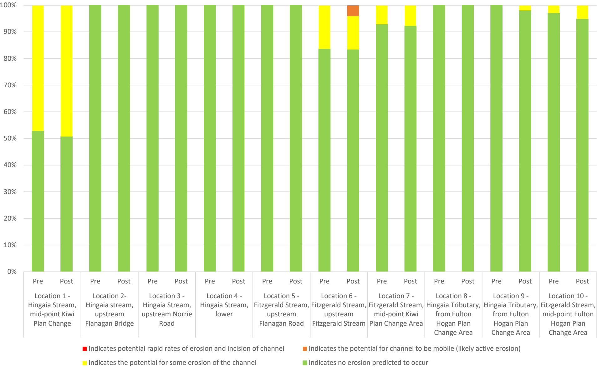
Excess shear stress in streams during 2 Year Pre and Post Development MPD CC
