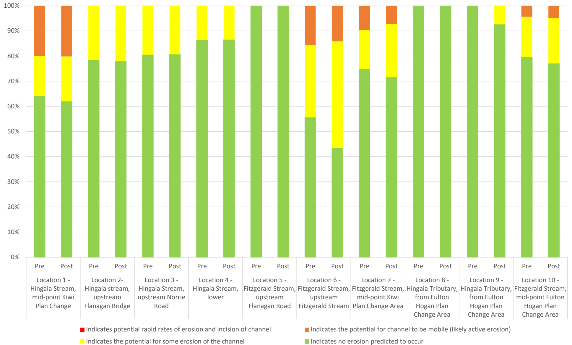
Excess shear stress in streams during 10 Year Pre and Post Development MPD CC
