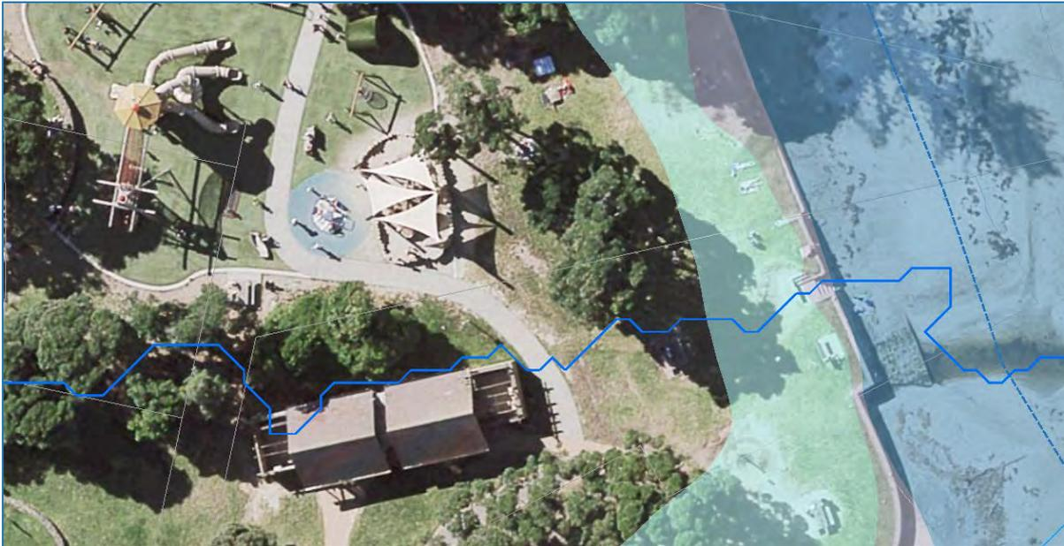
Figure 9: GeoMaps of southern accessway area showing Overland Flow path and various Coastal Inundation 1% AEP models: 1% AEP = blue shading, 1% AEP + 1m Sea Level Rise = grey shading, 1% AEP = 2m Sea Level Rise = turquoise shading..
