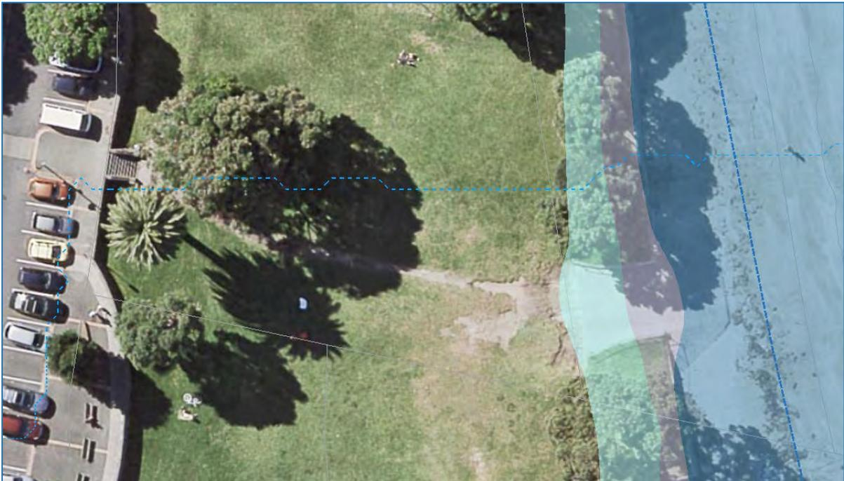
Figure 8: GeoMaps of northern accessway area showing Overland Flow path and various Coastal Inundation 1% AEP models: 1% AEP = blue shading, 1% AEP + 1m Sea Level Rise = grey shading, 1% AEP = 2m Sea Level Rise = turquoise shading.
