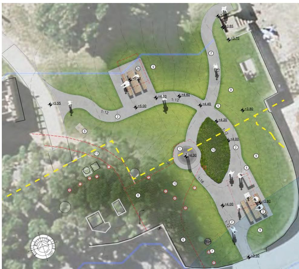
Figure 3: New accessible path layout soon to be constructed.
