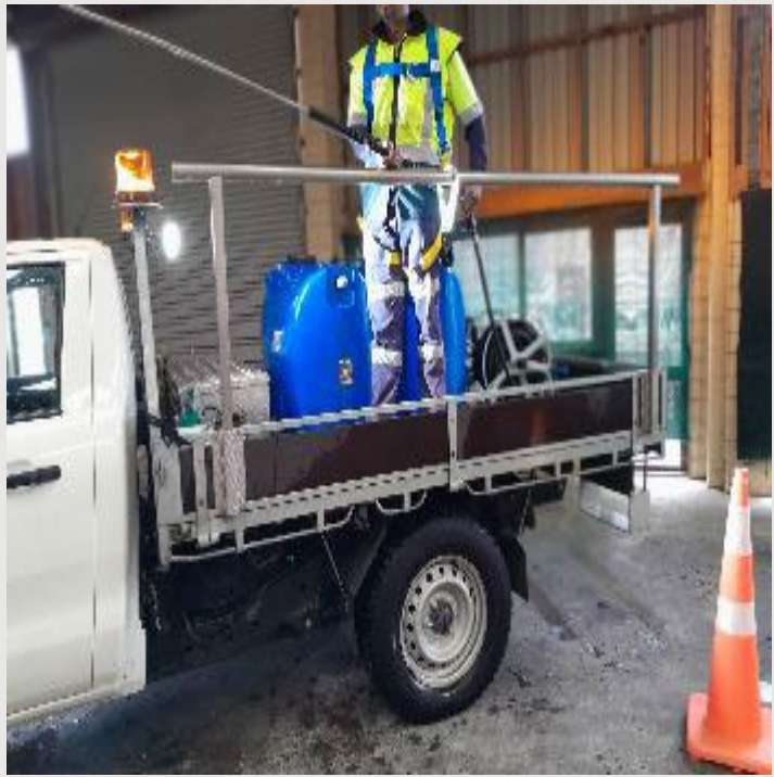
Outfitted the rear section of our water-blasting ute with sturdy safety rails
