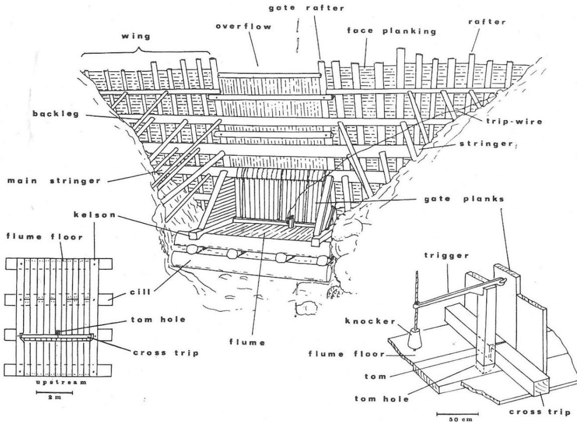
Figure 119. Sketch of the large dam on the Kaiarara Stream (now destroyed) showing the various parts of the structure. The dam is unusual in that three layers of sills were used below the flume. (Diamond and Hayward n.d. p16-17)
