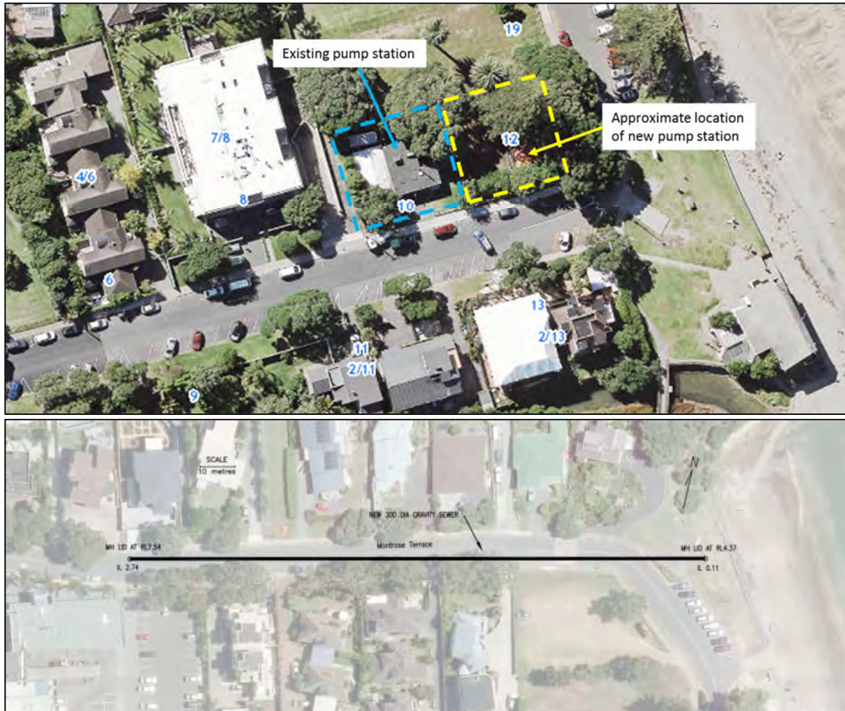
Figure 2.8: Location of proposed Mairangi Bay Pump station and gravity sewer
