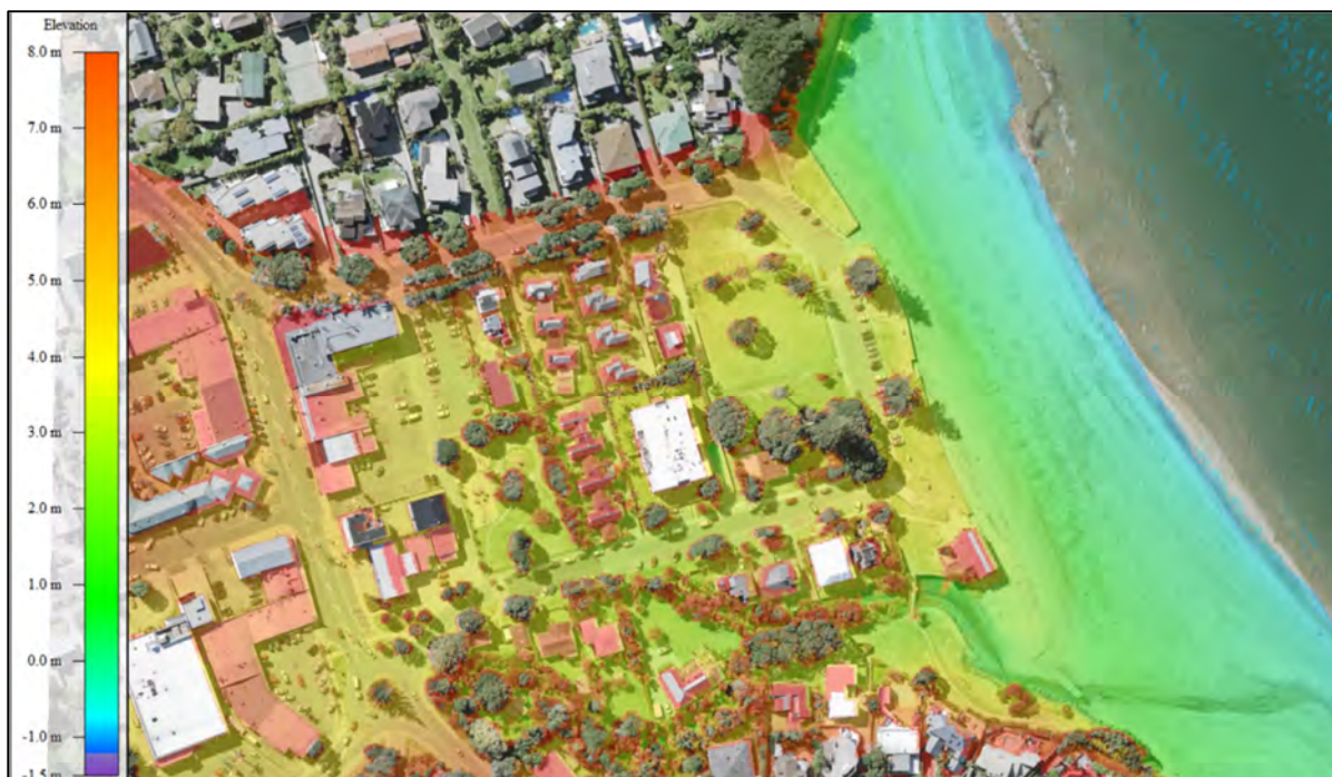
Figure 2.3: Local topography surveyed in December 2016, with elevations relative to AVD-46 (Auckland Council 2016-2017 LiDAR)
