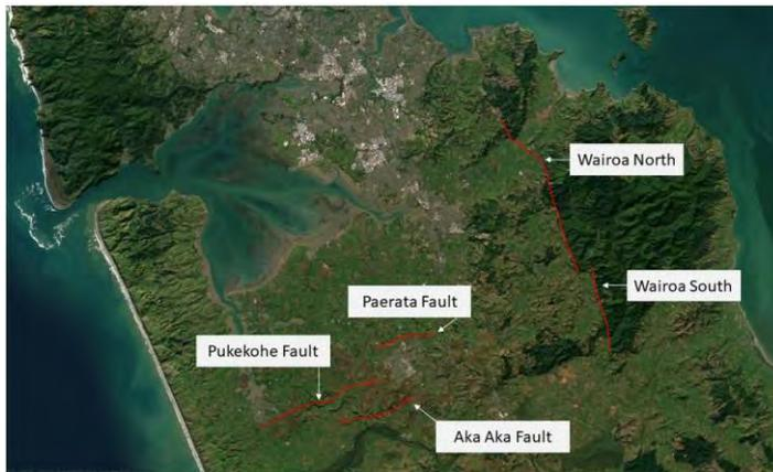
Figure showing faults within the Auckland region (note that the Paerata, Pukekohe and Aka Aka Faults require more research to understand their risks, as recent mapping has just recently identified these features).
