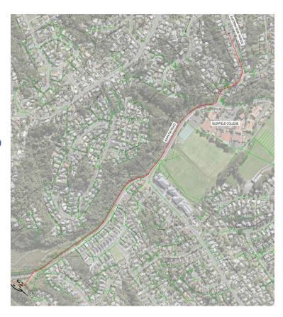
Diversion of connections for existing Kahika Transmission pipeline so it can be decommissioned
