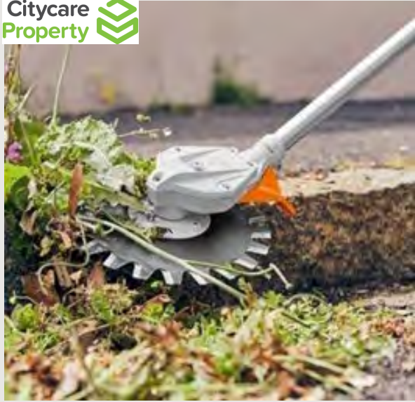
Weed eater Attachment Trials to reduce stone chip incidents
